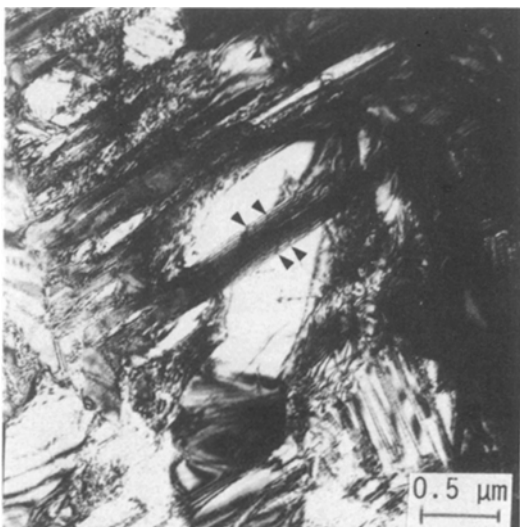
Figure 6 TEM of \langle 123 \rangle crystal [13], T = 700^{\circ}\text{C} , \epsilon = 0.015 . Foil is normal to \langle 123 \rangle .
